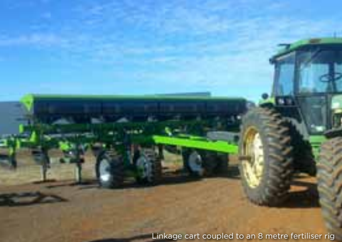
Linkage cart coupled to an 8 metre fertiliser rig
