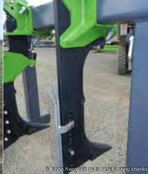
6 Row - 3 Bar Side Buster being used to knock down rotor bucks
